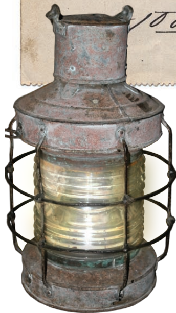
An early 1900s riding light from a schooner was hoisted in the fore-rigging during the night while the boat was anchored.
